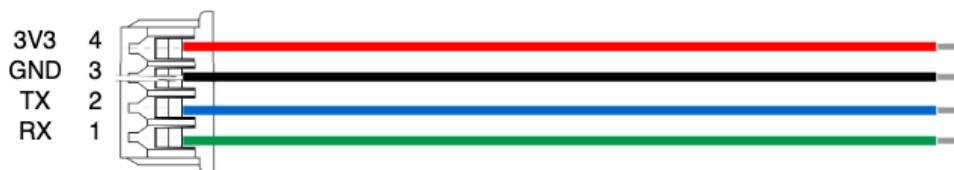
Figure 20: UART cable diagram
