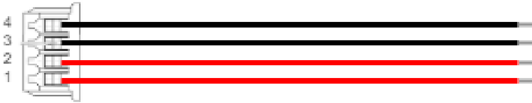
Figure 6: Voltage input cable pinout for Molex PicoBlade (red = V+, black = GND)
