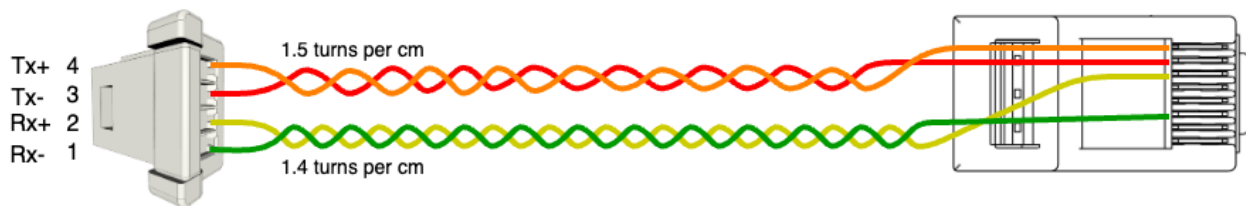
Figure 11: Ethernet cable pinout for Molex PicoClasp variant
