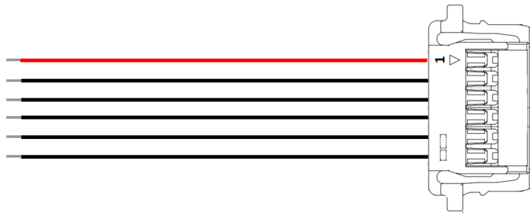
Figure 18: LED breakout cable diagram
