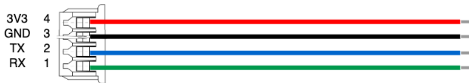
Figure 20: UART cable diagram
