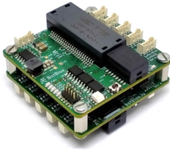
Figure 13: Back to Back operation (two SwitchBlox Rugged)
