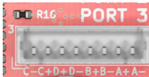
Figure 6: Ethernet port pinout
